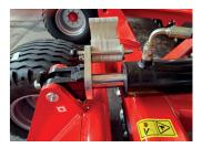
Working depth up to 18 cm The working depth is adjusted by means of clips on the individual hydraulic cylinders and controlled by a single hydraulic circuit. The machine can thus be quickly and easily adjusted to suit the conditions.
